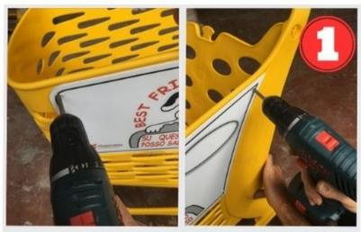
Use a fibreboard as a template to drill the holes with a 6 mm drill bit
